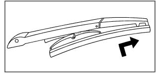
5. Remove clip (B), shown in step 3, and slide it into the remaining claw of the wiper blade assembly.
